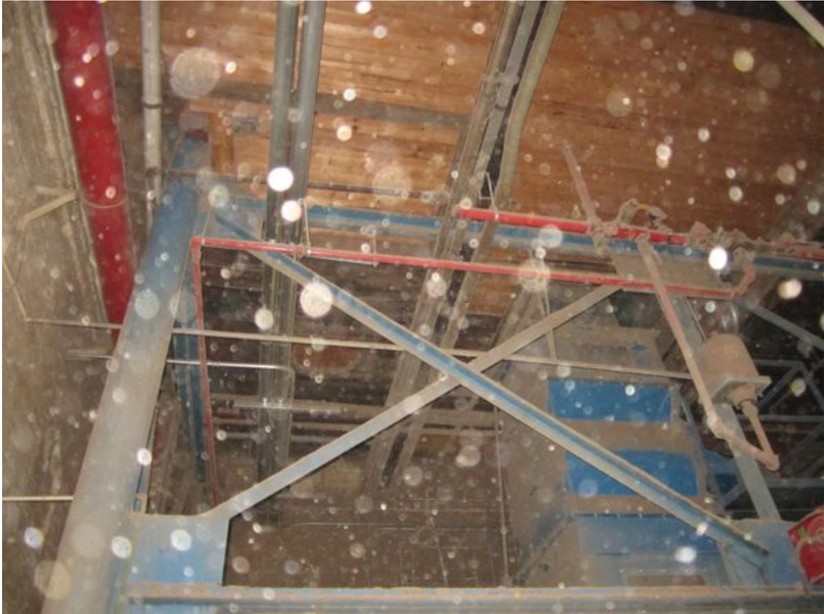
*The above image shows airborne dust particles created by a closed loop dust collection system. The little spots are dust particles reflected in the camera flash. At G.F. Puhl, we call this a "dust bomb" because of the explosion risk created by airborne dust particles.*
